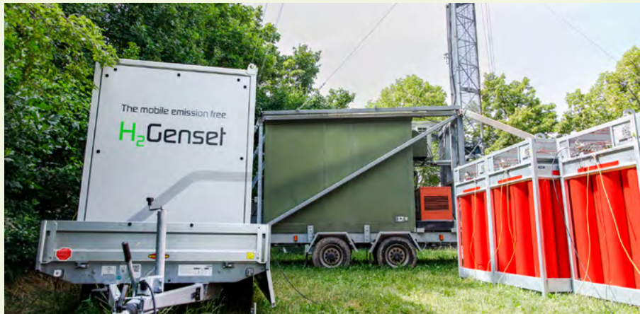
An emission-free generator, the 'H2Genset', Test-Fuchs GmbH
